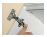
Mount the hinges of the fixed door onto the mounting plates on the cabinet side. We recommend the use of SALICE hinge 329.17.600 with mounting plate 329.71.500 or similar.
